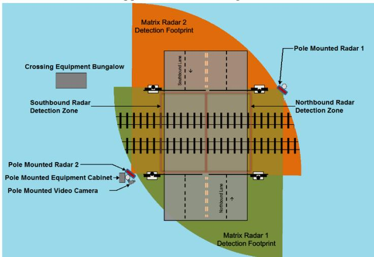
Figure 4: Layout of radar detection system at the crossing island (Island Radar).
