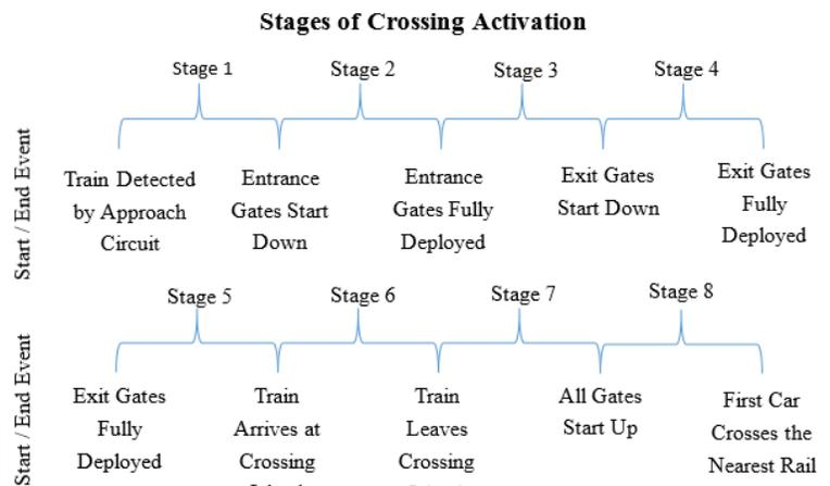
Figure 5: Stages of crossing activation based on operational events.
